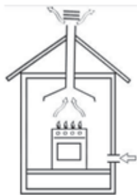
In a chimney stack or branched flue.
