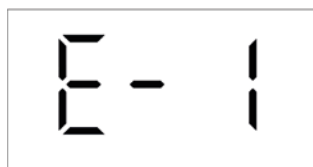
Pic 11: Sensor abnormal alarm display effect
