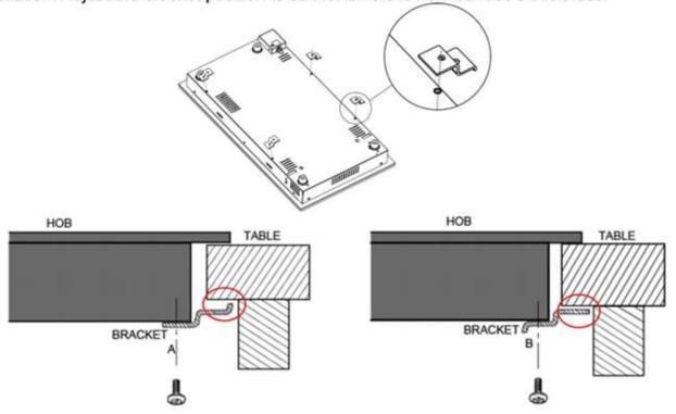
Under any circumstances, the brackets cannot touch with the inner surfaces of the worktop after installation (see picture).
