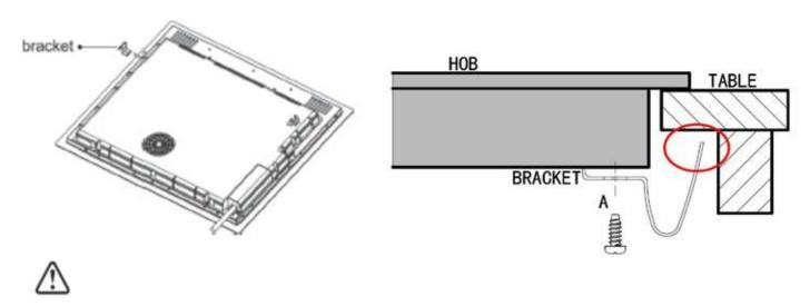
Under any circumstances, the brackets cannot touch with the inner surfaces of the worktop after installation (see picture).
