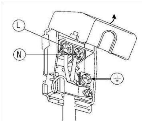
***Connection of the power cable to the mains.***
