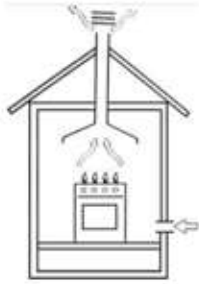
In a chimney stack or branched flue.
